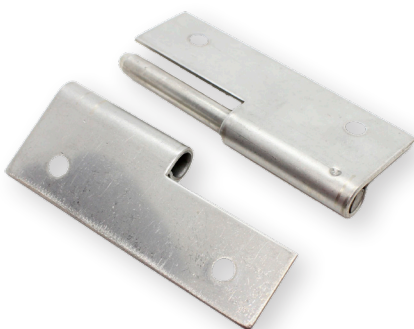
304 Stainless Steel Lift Off Hinge 50mm x 76mm x 1.5mm 5mm Mounting Holes, 6.35mm Thick Pin
